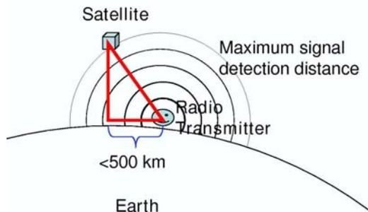
**Figure 3.** The proposed system for approximate location of radio signals transmitted from a ground-based transmitter [see also 5].
